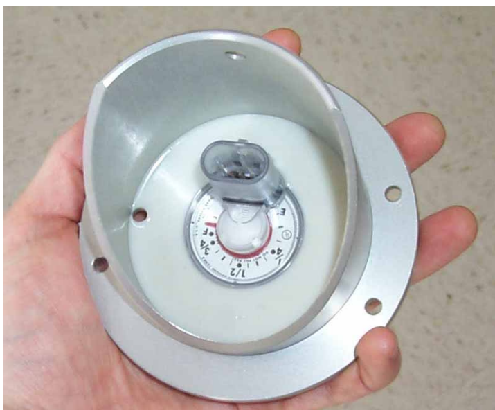
Figure 3: Float gauge magnetic-coupler
