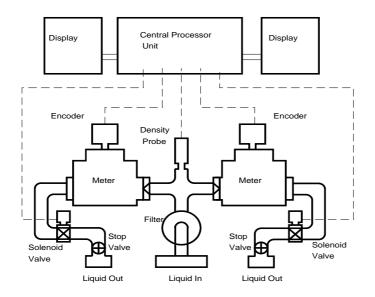
Liquid enters the dispenser through the filter and then passes over the vapour sensing probe and enters the meter through a soft seat back check valve. The liquid leaves the meter and passes through a delivery control solenoid valve, a manual stop valve, excess flow valve, hose, line break and dispensing nozzle.
