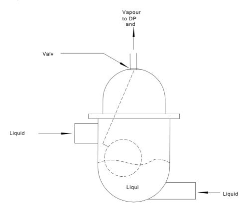
If a large amount of vapour is present in the system, the float will fall and the vapour will exit through the top of the vapour eliminator. This vapour will return to the tank and may be used to provide high pressure to the Differential Pressure (DP) valve to stop delivery while the vapour is being cleared.
